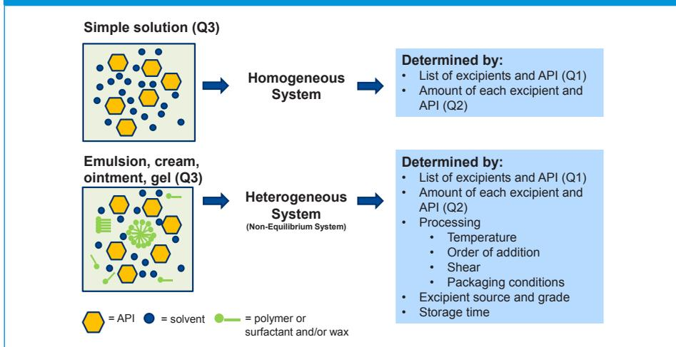
So it is not just the list of ingredients, but it is how all of these ingredients interact and the phases that they form that drives the performance criteria. The structures that form will affect the viscosity, stability, and sensory, as well as API solubilization, the API release, and the API absorption.
