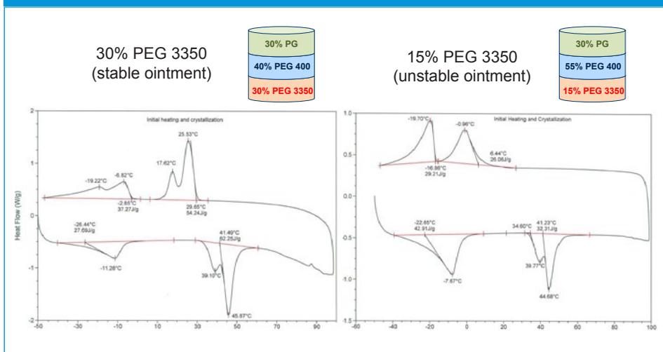
**Figure 11:** Variations of Solid (PEG) Phase and Concentration – Solid Phase and Concentration exhibit clear effect using XRD
