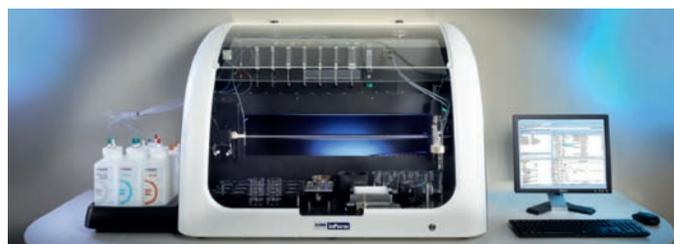
Figure 2: Pion InForm® utilized for measuring precipitation kinetics in this study
